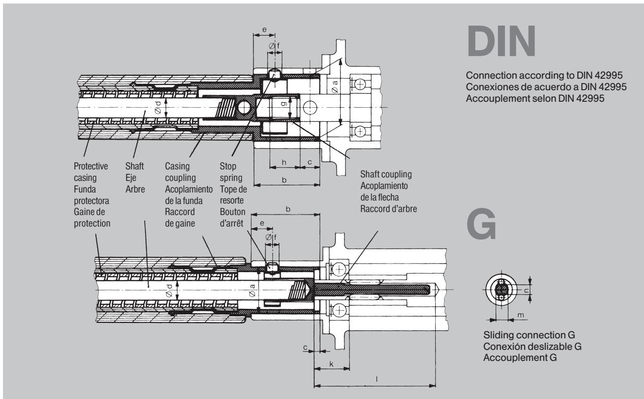
For connecting flexible shafts to the machines and accessories, two coupling systems are available:
